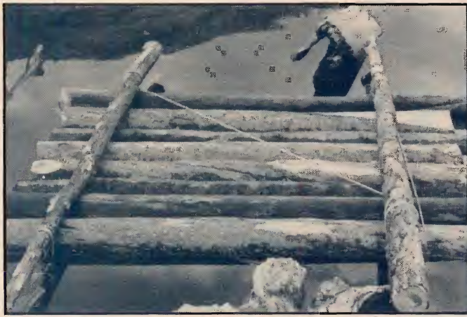
ABOVE — The pressure bar raft can be constructed with a 50-foot rope.
